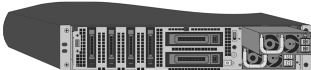
Figure 1-14. Inserting the Replacement DC Power Supply
